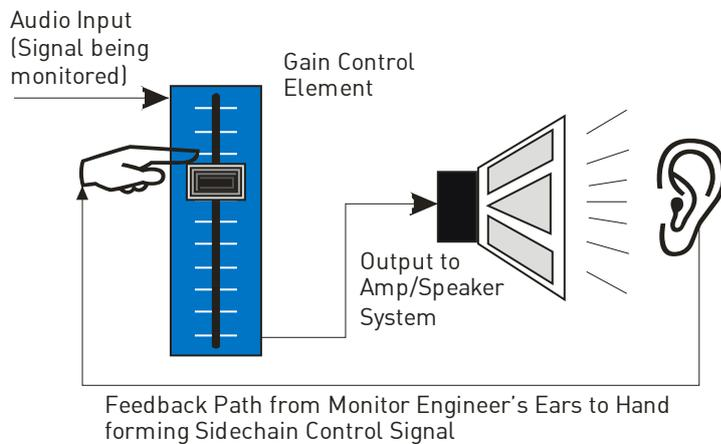
There is a hidden sidechain in operation even in this case. The main signal path is fed through the monitor desk and the gain controlled by adjusting the fader. The sidechain is formed by the feedback path between the engineer's ears checking the level and his brain instructing his hand to turn the fader down if the volume goes over the threshold he has chosen.
