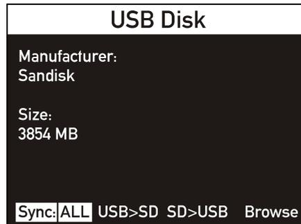
To copy the firmware from the USB stick onto the amplifier's SD card, use the encoder to highlight the USB>SD option, and press ENTER. Any files in the /firmware folder on the USB flash drive that are not already in the corresponding folder on the SD card (with the file extension ".bin") will be copied, and the progress will be shown:
