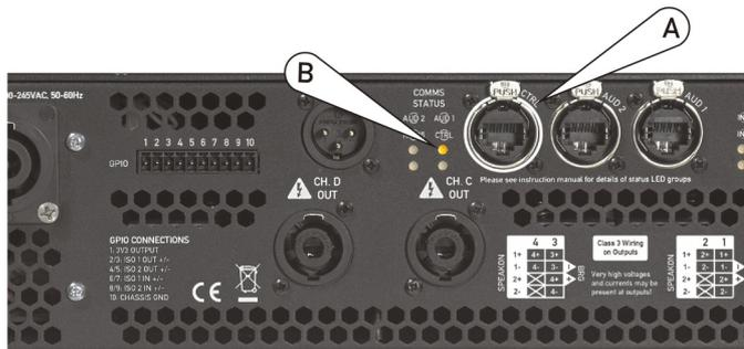
Plug a standard Ethernet cable into the “CTRL” port on the rear of your APA (A).
