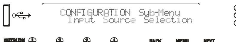
Use the encoder or BACK and NEXT keys to find the Input Source Selection option and press ENTER.
