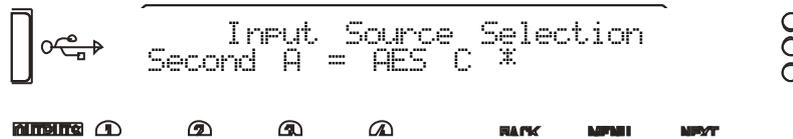
Use the encoder or BACK and NEXT keys to scroll through the eight choices for this input. Selecting an analogue source as the secondary will finish the selection process for this input and move onto the primary choice for the next input. If a digital source is chosen for the secondary, then a final step will determine if the tertiary (final) failover source, which can only be analogue is to be used:
