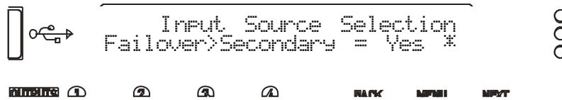
Use the encoder or BACK and NEXT to select Yes if you wish this input to use the Failover system and automatically switch to your secondary input source, should the primary fail. Press ENTER.
