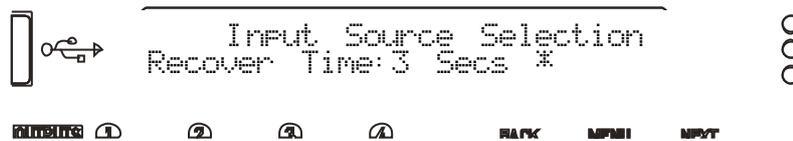
Use the encoder or BACK and NEXT keys to select the time for the system to hold before reselecting the higher order source. It is possible to prevent the higher order source taking over again by selecting "Never" from the list. Press ENTER to confirm the changes and exit to the home screens.
